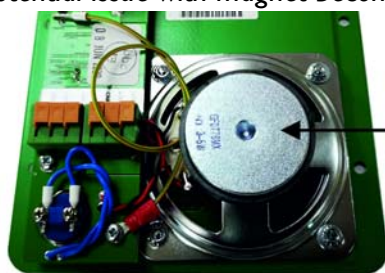
Figure 1 — Potential issue with magnet becoming loose or detached (C2RRG shown)
