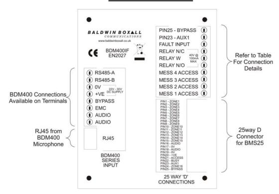
The BDM400IF allows a BDM400 microphone to be retro-fitted to an existing system through a BMS25 termination unit using a 25way D type cable.
