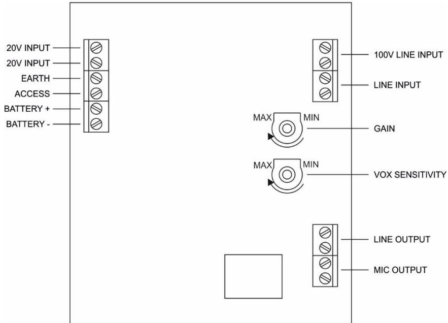
**Figure 1 – BT10 Controls and Connections**
