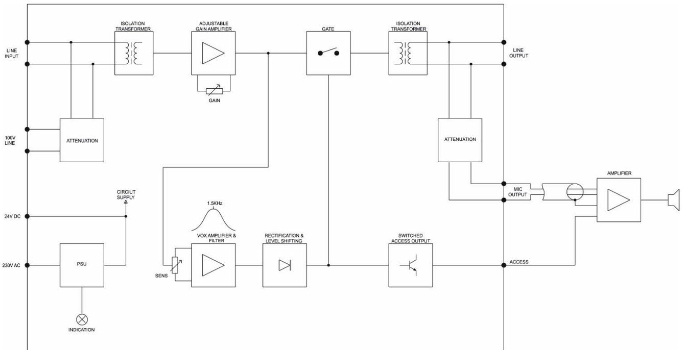
**Figure 2 – BT10 Functional Block Diagram**
