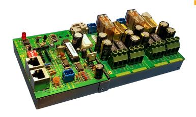
The DC line monitor isolator units are CANBUS modules for the VIGIL voice alarm systems with VIGIL3 amplfication, consisting of two components: BV3ADIM and BV3ADIS
