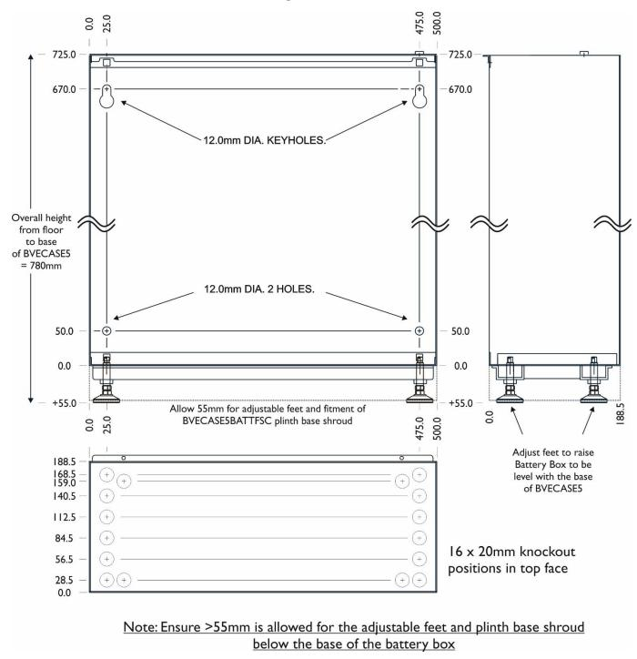
Note: Ensure the internal battery mounting plinth is fitted to the base of the battery box before installing the batteries.
