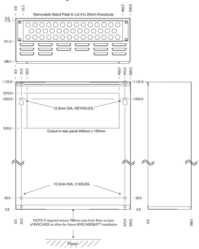
Note: The BVECASE5 has been designed to allow cable entry from the top (via knockouts) or via the removable access plate in the rear panel.
