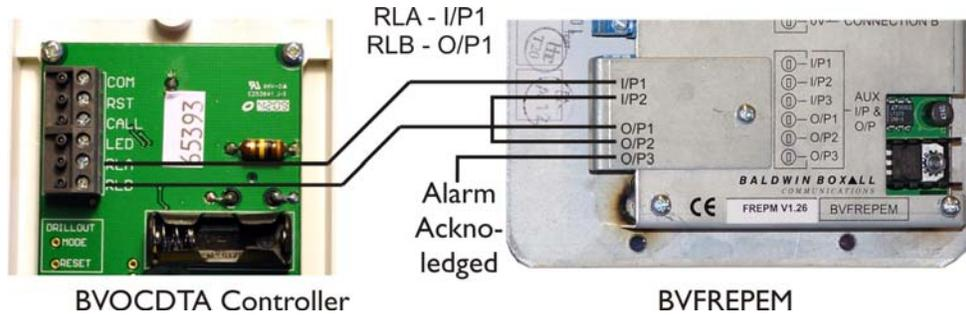
Note: The BVFREPEM includes a Normally Closed Fault Input between I/P 2 and O/P 2. These points must be linked to prevent a fault being announced.
