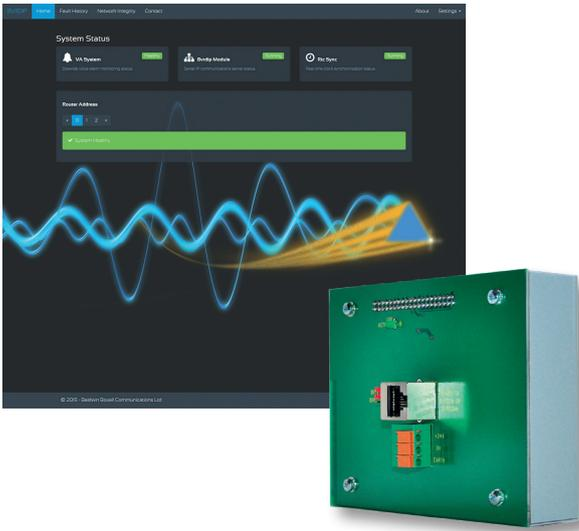
The BVRDIP interface enables a connection from VIGIL systems to an IP network, such as LAN or internet. This allows for remote monitoring of your voice alarm system via internet connected devices.
