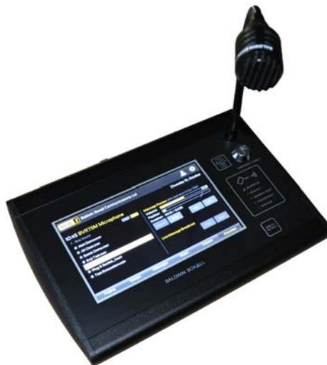
The Microphone is configured during commissioning using the built touchscreen. Standard RJ45 Network cable connections (carrying both Audio and Serial Data) are employed, in order to make installation simple and flexible.
