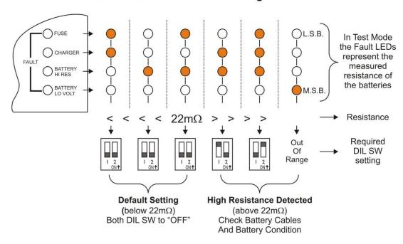
Set the front panel DIL SW to match the detected resistance.
