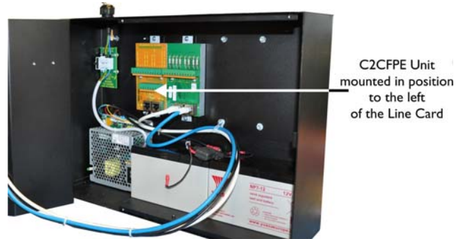
Figure 2.12 — Internal View - C2CFPE unit mounted in position
