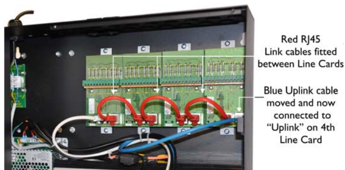
Figure 2.9 — Console with Four Line Cards Fitted
