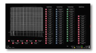
OmniCare is an addressable voice communication system that allows disabled refuge, fire telephones, emergency/steward telephones and disabled toilet alarms to be connected to one master panel. Touchscreen control adds further flexibility to the system.
