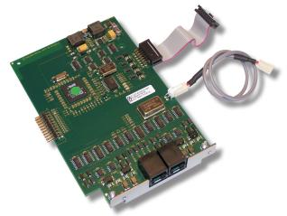
The BVRDNET2M4 provides a digital networking solution for the OmnicarePLUS emergency voice communication system.
